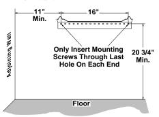
Figure 13 - Mounting Bracket Clearances
